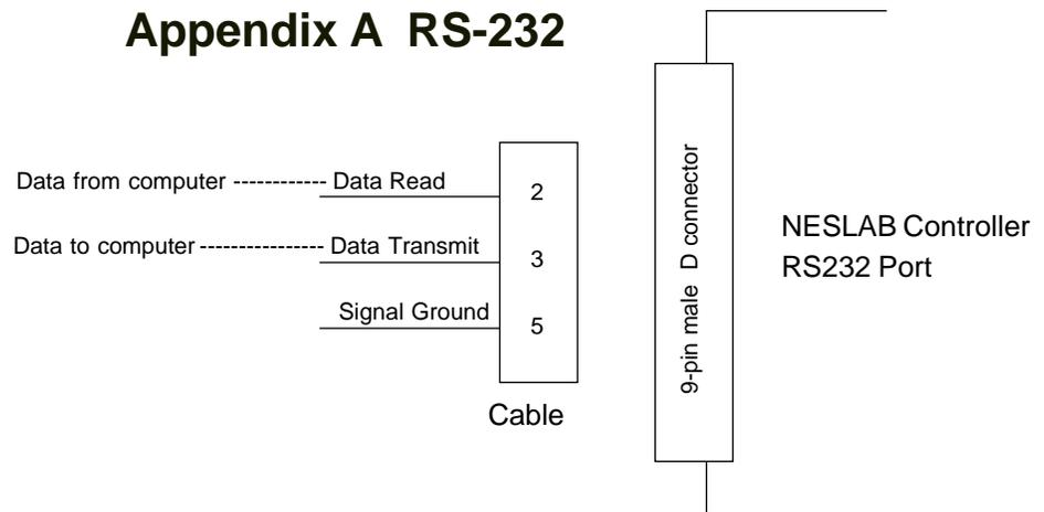
The unit can be controlled through your computer's serial port by using a standard 9-pin RS232 connection on the rear of the temperature controller. Data transmit of the serial port connects to data read (pin 2) of the bath. Data read of the serial port connects to the data transmit (pin 3) of the bath.
